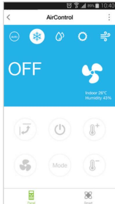
After you've connected, you'll see the room temperature on the AirControl screen and a new device in the **Device list** of the app.
