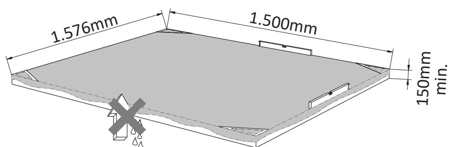
[EN] Laying on concrete slabs (not included)
