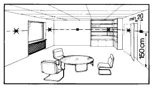
The unit can be fitted to a recessed conduit box or directly on the wall.
