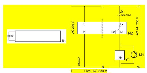
N1 Thermostat (RDE100.1/RFS-EQ) No wiring is required as thermostat is battery operated.
